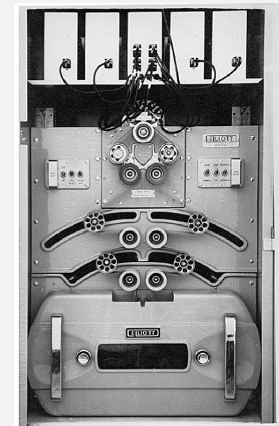
Elliott 405 magnetic disc (16K words)
