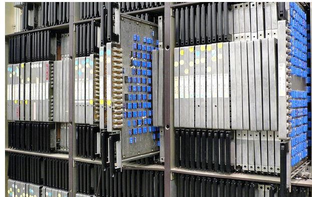
ILLIAC IV Processing Unit and Control Unit https://en.wikipedia.org/wiki/ILLIAC_IV
